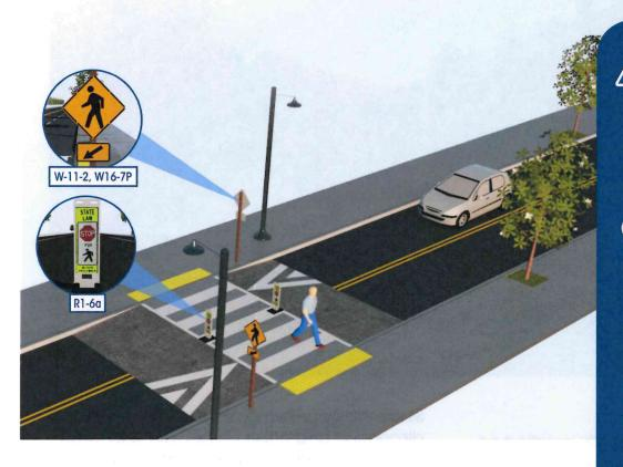
Raised crosswalks are ramped speed tables spanning the entire width of the roadway, often placed at midblock crossing locations. The crosswalk is demarcated with paint and/or special paving materials. These crosswalks act as traffic-calming measures that allow the pedestrian to cross at grade with the sidewalk.
